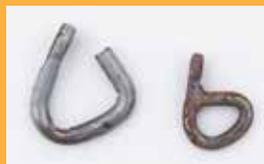
shuts, open and closed, and both are dangerous. Many cold shuts were welded in a climber's garage. Explaining the danger of that, Sandor Nagay wrote in *Climbing* magazine, "None of us would climb on a rope that our buddy wove in his garage, but many of us trust cold shuts implicitly."
