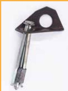
**LEEPER HANGERS:** These hangers are easy to identify by their typically blackened color and semi-sharp edges, compared to the rounded shape of a modern hanger. Leeper hangers were the first commercially made hanger designed specifically for climbing and eventually were recalled.
