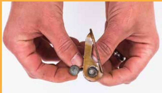
**STAR DRYVINS:** Typically called star drives, these bolts can be identified by the star stamped on their heads. Star drives tend to have a greater degree of variability in terms of how bomber they are, but they have been known to come ripping out of the wall with a quickdraw yank.
